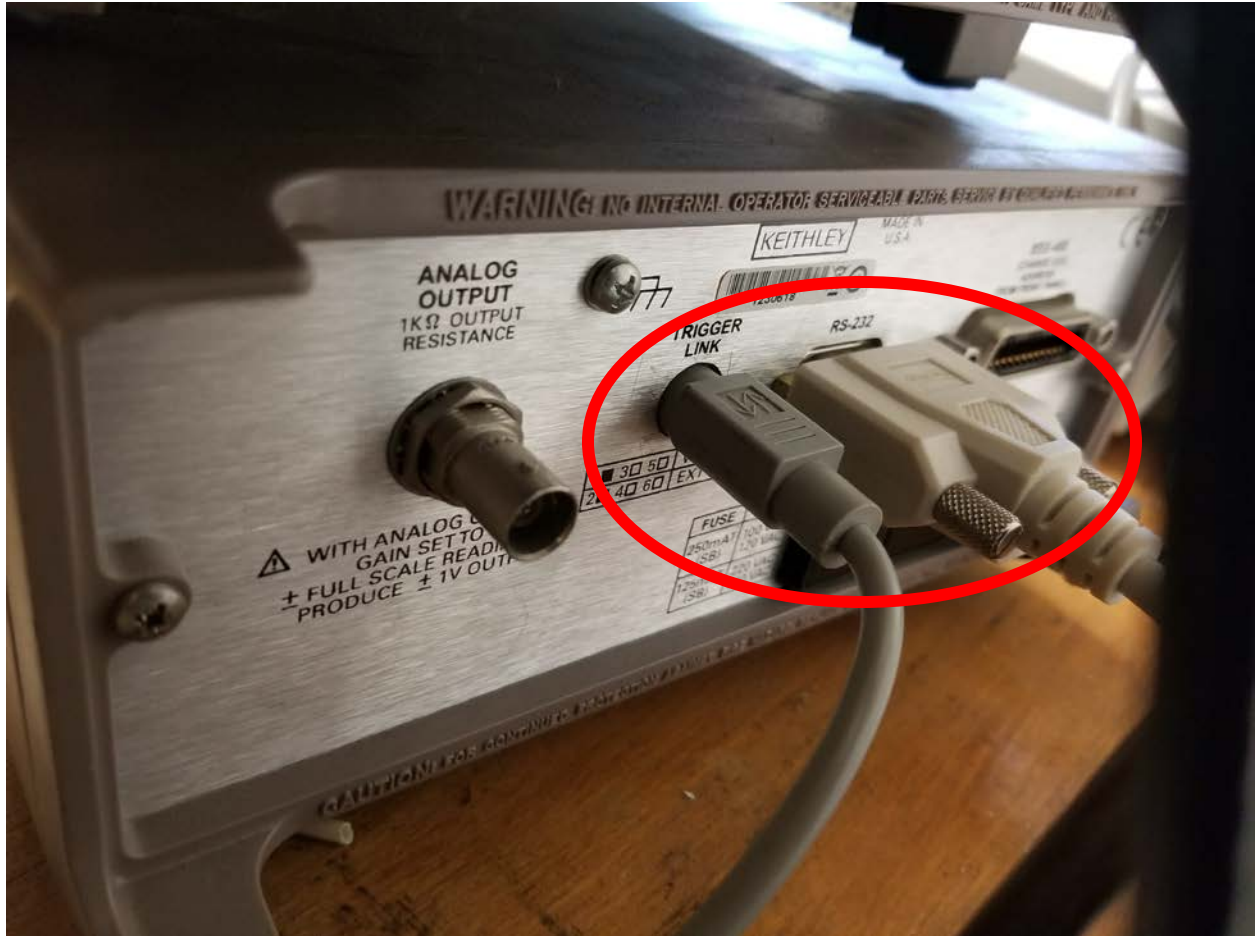
Back of the Keithley 2182 voltmeter box. RS232 cable on the right, Trigger Link cable on the left. The back GPIB cable is disconnected.
